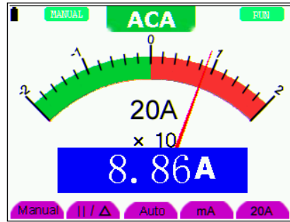
Figure 30: AC Current Measurement for 20A
